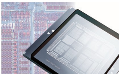
A photomask used for manufacturing semiconductors
