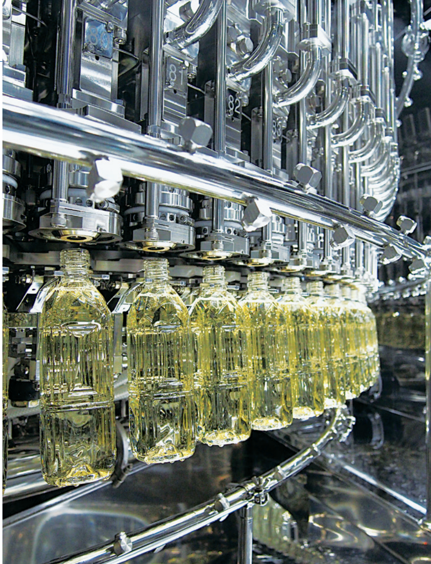
DNP Aseptic Filling system for PET bottle for CSD and Non-CSD Up to 60,000 bph
